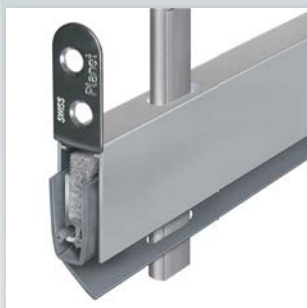
Option: Planet RH with Planet drill hole \varnothing 5 \times 13 mm and driving bar rod → refer to chapter Accessories | driving bar rods
